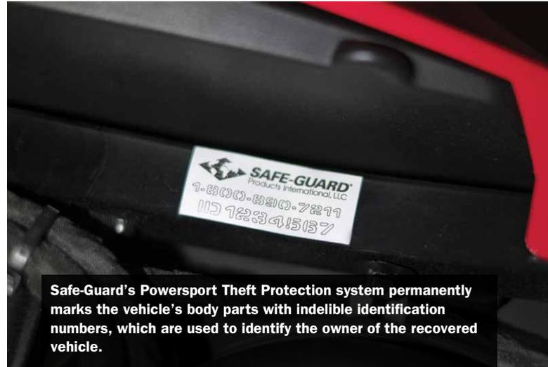
Safe-Guard's Powersport Theft Protection system permanently marks the vehicle's body parts with indelible identification numbers, which are used to identify the owner of the recovered vehicle.
